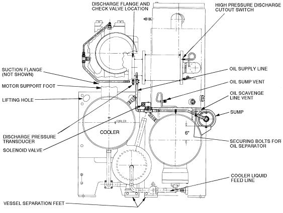
Fig. 8 — 23XL Drive End View (Frame 1 and 2 Machines)
